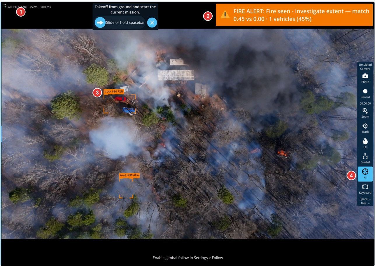
Figure 5.1 — Detection boxes and a fire alert.
